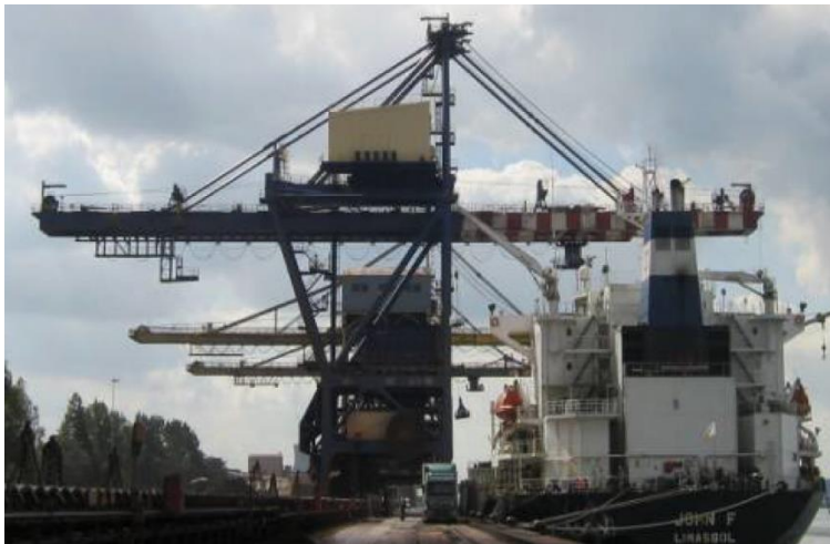
Figure 1: The Arcelor Mittal Gent bulk material quay. Five large portal cranes can discharge two Panamax bulk carriers and one barge simultaneously. The coordination of the discharging activities will be scheduled by the quay planning heuristic.
